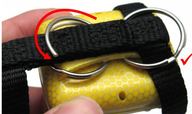
The picture shows how the two rings mount the tracking device to the harness.
