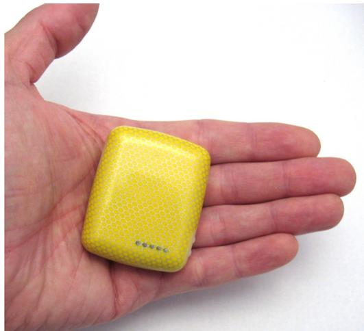
Turn on the unit outdoors by pressing the “on/off” button until the indicator light is on. For first use, please initialize the unit and restore it to default setting (please refer to next section for instructions). After about 50 seconds the unit will begin to work and acquire the GSM signals as well as the GPS signals.
